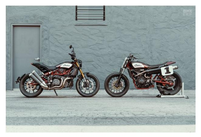
The seat is also bigger than the perch on the concept bike, with passenger pegs down below, and the back wheel has gone down a size from 19 to 18 inches.
