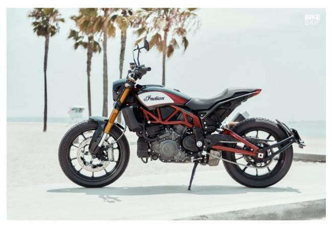
There's a new 1203 cc engine that pumps out 120 hp, an under-seat tank for mass centralization, and a trellis-style steel mainframe with an aluminum rear subframe.
