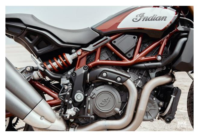
The power peak is 120 hp at 8250 rpm, and 85 ft-lbs (115 Nm) of torque is delivered at 6,000 rpm. According to Indian's press pack, "A flat torque curve ensures a progressive, predictable power delivery with loads of low-end punch and flexibility."
